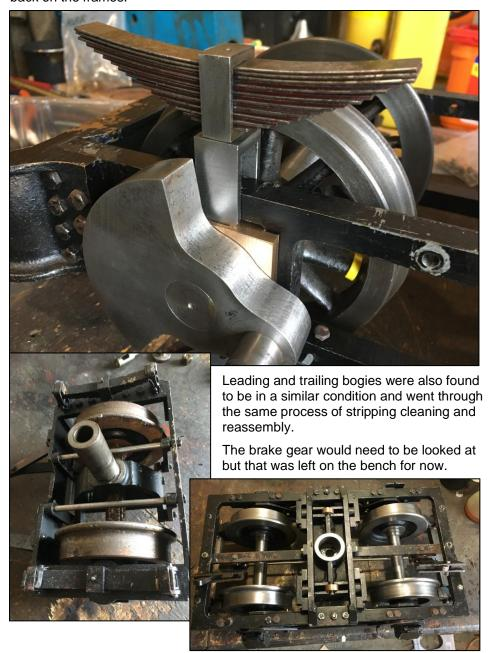
The next job was inspection of the cylinders and steam Which chests. were found to be in an acceptable condition and so after the now usual clean up were reattached the to frames. And the slide valves and pistons were refitted.
